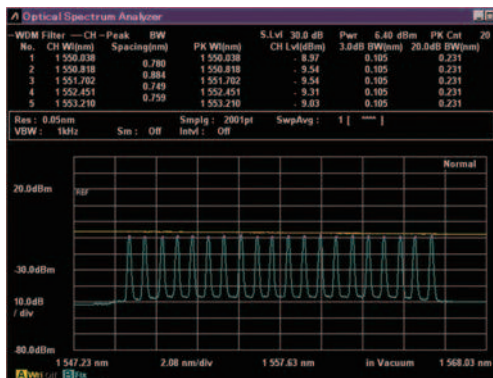
Waveform of Wideband Light Source Before and After Insertion to Optical Bandpass Filter
